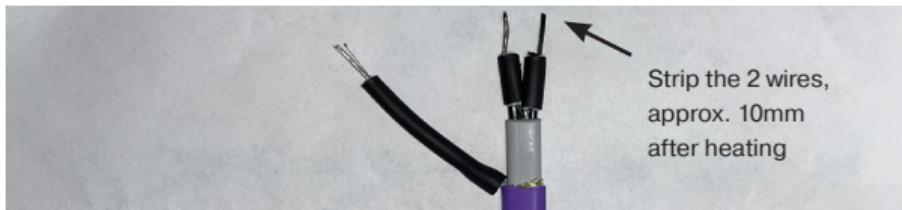
Install shrink tubing 12/3x17mm over the middle insulation and heat
