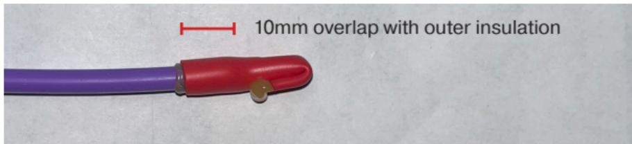
Install end cap 14/5x55mm, heat and push back with pliers until it cools down
