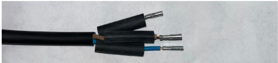
Crimp the ferrules onto the heating cable conductors and heat the shrink tubing.
