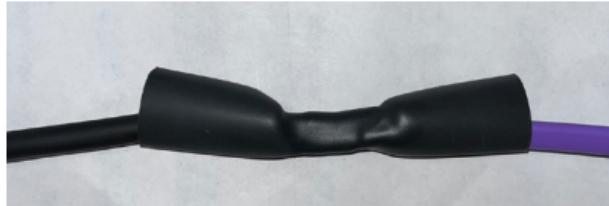
Center the shrink tubing 19/6x200mm over the connections and heat from the center and outwards
